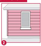
Install non-combustible siding (stucco, metal, stone, cement fibre board).
