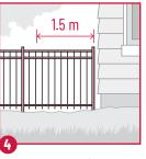
Install non-combustible fencing within 1.5 m of the house (cement fiber, metal, chain link or stone).
