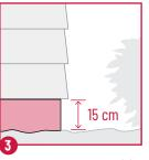
Create a 15 cm ground-to-siding non-combustible clearance (e.g., install cement board or metal skirting).
