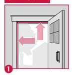
Replace worn or missing weather stripping on all doors including garage doors.
